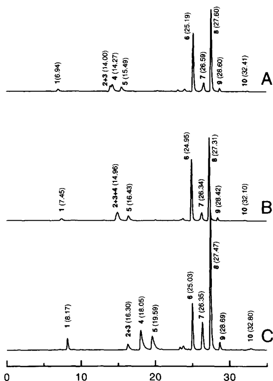
Fig. 3. Chromatograms of chlorophyll standards on the polymeric ODS column (Vydac 201 TP) using mobile phases containing (A) pentylamine, (B) piperidine and (C) pyridine. Peak identification as in Fig. 2. Retention times are indicated in brackets. For other chromatographic conditions, see Section 2.
